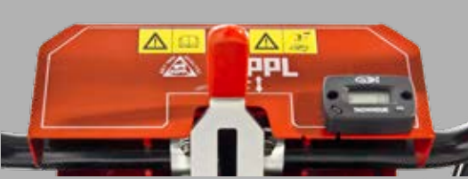
Tidy dashboard with operating hours meter and steering shaft height adjustment
