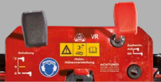
Well-arranged panel with handlebar height adjustment and gear shift diagram
