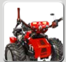
Rear view: Hydro Athlet-handlebar 180° rotated with 30° lateral offset
