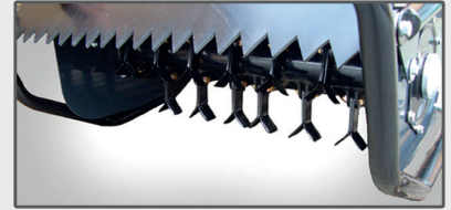
Cutting rotor with 38 blades
